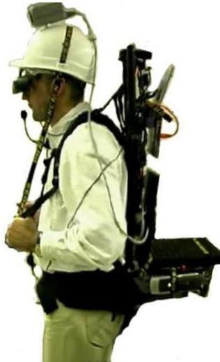
Figure 7.1: A side view of our prototype wearable computer built with DWARF.
